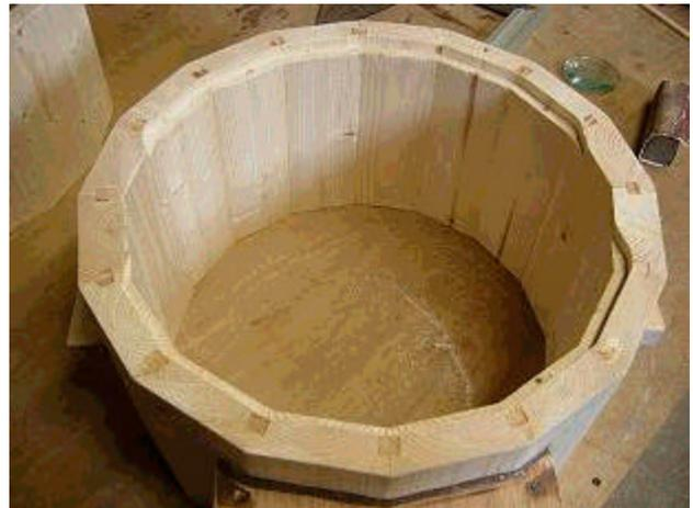
The end grain is rubbed down with sandpaper to improve paint adhesion.
